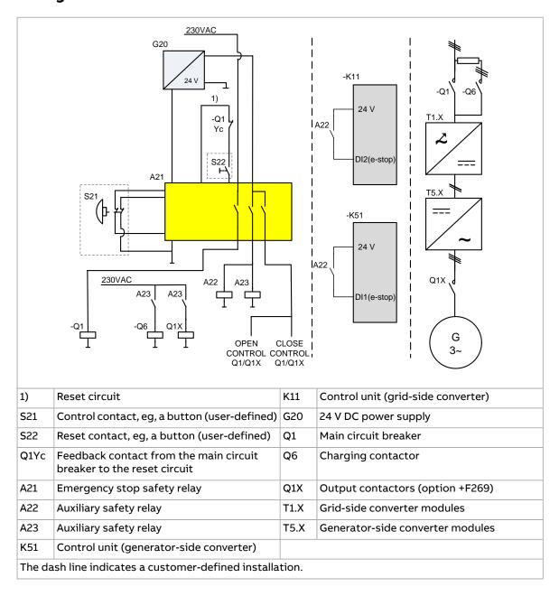
Initial status: The converter is running and the wind turbine is rotating. In this example, the user gives the emergency stop command and resets the emergency circuit with buttons.
