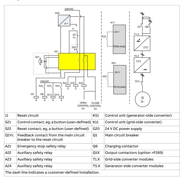
Initial status: The converter is running and the wind turbine is rotating. In this example, the user gives the emergency stop command and resets the emergency circuit with buttons.
