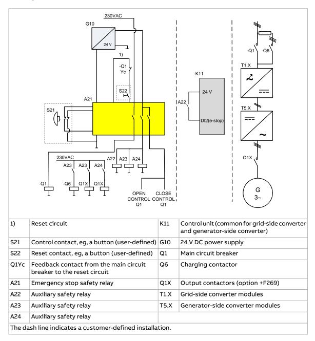
Initial status: The converter is running and the wind turbine is rotating. In this example, the user gives the emergency stop command and resets the emergency circuit with buttons.
