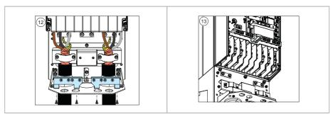
15. Ground the motor cable shield at the motor end. For minimum radio frequency interference, ground the motor cable shield 360° at the lead-through of the motor terminal box.
