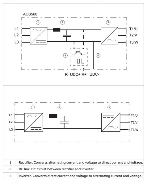
Built-in brake chopper (R-, R+/UDC+, UDC-) in frames R0...R2 and (R-, R+) in frame R3. Conducts the surplus energy from the intermediate DC circuit of the drive to the brake resistor when necessary. The chopper operates when the DC link voltage exceeds a certain maximum limit. The voltage rise is typically caused by deceleration (braking) of a high inertia motor. The user obtains and installs the brake resistor when needed.
