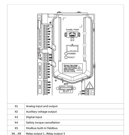
Option slot 1 (fieldbus adapter module)
