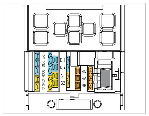
Connect the external supply or module to the +24V and DGND terminals (40 and 41).
