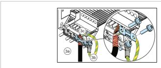
Tighten the screws to the torque given below.
