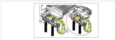
9. Tighten the screws to the torque given below.
