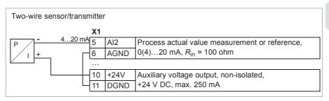
**Note:** The sensor is supplied through its current output and the drive feeds the supply voltage (+24 V DC). Thus the output signal must be 4...20 mA, not 0...20 mA.
