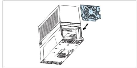
4. For IP21 (UL Type 1): To install the auxiliary fan, refer to Replacing the auxiliary cooling fan, IP55 (UL Type 12) frames R1 ...R2 or Replacing the auxiliary cooling fan, IP55 (UL Type 12) frame R3 in the hardware manual.
