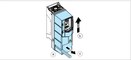
6. For R4 and R5: Attach the U-brackets (b and c) to the back of the drive.
