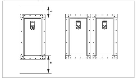
**Note:** The free space requirements below are for the heatsink side of the mounting plate. There is no free space requirement for the front side of the mounting plate. That area can be occupied by other equipment (for example, contactors, relays, wires, ducts, and so on).
