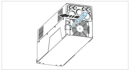
2. For R4, IP21 (UL Type 1): Insert the sealing plug (a) into the hole.
