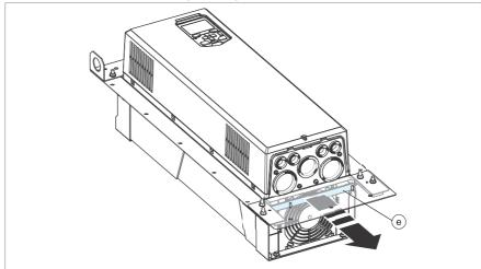
11. For R4 and R5: Remove the tightening bracket (e) from the front of the fan.
