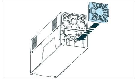
3. For R4, IP21 (UL Type 1): Install the fan assembly.
