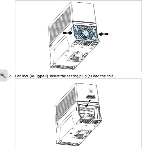
3. For IP21 (UL Type 1): Install the fan assembly.
