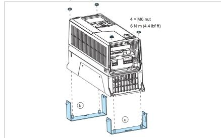
6. Attach the U-brackets (b and c) to the back of the drive.
