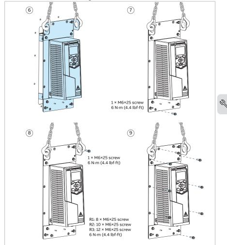
34 Mechanical installation – Frames R1...R3
