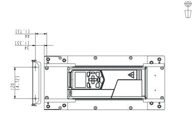
The hood is needed for UL Type 12 installation only.
