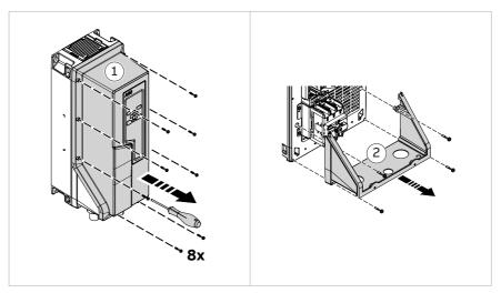
3. Install the flange onto the drive frame.
