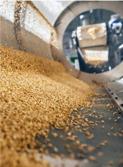
01 VSD/VFD provides precise speed and torque control of milling rolls to ensure that grain is milled consistently and to the required quality.
