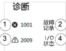
The screenshot shows a menu titled '诊断' (Diagnosis) with four numbered callouts: 1 points to a crossed-out circle icon next to '1001', 2 points to the text '故障记录' (Fault Record), 3 points to a warning triangle icon next to '2009', and 4 points to the text 'I/O 状态' (I/O Status).
