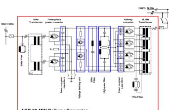
ABB 20-MW Railway Converter
