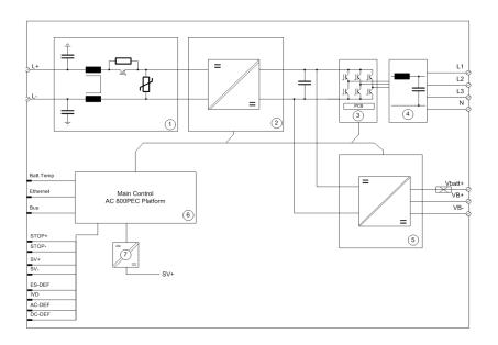
Block diagram for BORDLINE® M55 DC 750V
