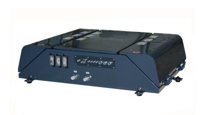
The Compact Converter BORDLINE® CC400 DC converts 600 Vdc or 750 Vdc line voltage into propulsion power to control and drive the traction motors and auxiliary power to supply the onboard loads. It is complemented by a modular energy storage system, including batteries, cooling and battery management system.
