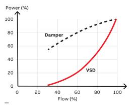
Figure 1: Graph showing fan power requirements for damper and VSD.
