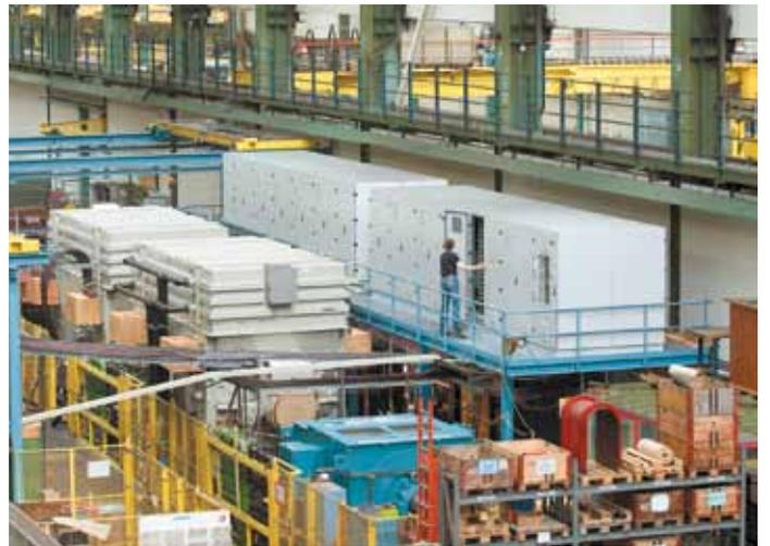
背靠背试验48 MW / 3,500 rpm
