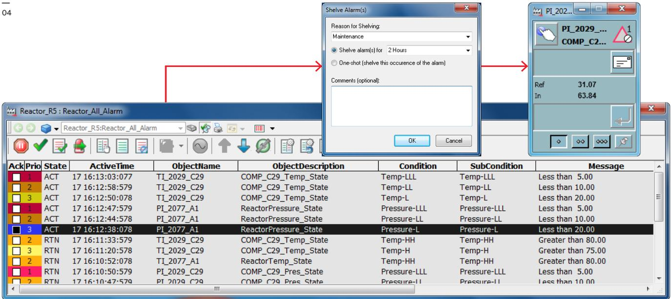
04 Alarm shelving helps the operators reduce distraction from nuisance alarms.
