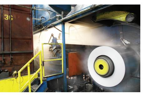
Jupiter Aluminum's three rolling mills are running with three Stressometer systems and six MTG thickness gauges.
