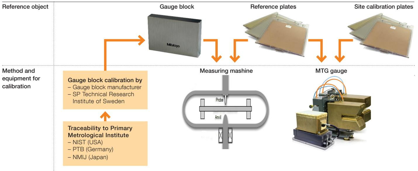
**MTG site plate calibration process**
