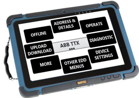
New ABB Field Information Manager (FIM) does offer all of this. It can be downloaded and installed within just a few minutes, offers access to meters using very common HART modems and state of the art FDI device packages representing the physical device like a printer driver. Legacy devices are supported by either a conventional EDD or by the integrated Generic Driver Package.
