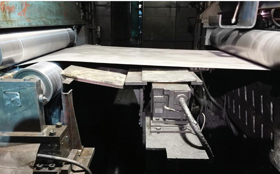
ABB's robust and reliable Millmate Strip Scanner systems are keeping track of the strip position at TISCO Stainless steel in Taiyuan China, one of the world's biggest stainless steel producers.
