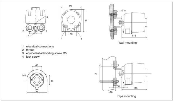
Fig. 3-2 Dimensional drawings of TF12/TF212 (all dimensions in mm)
