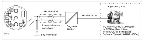
Fig. 3-4 Bus connection for communication and parameterization
