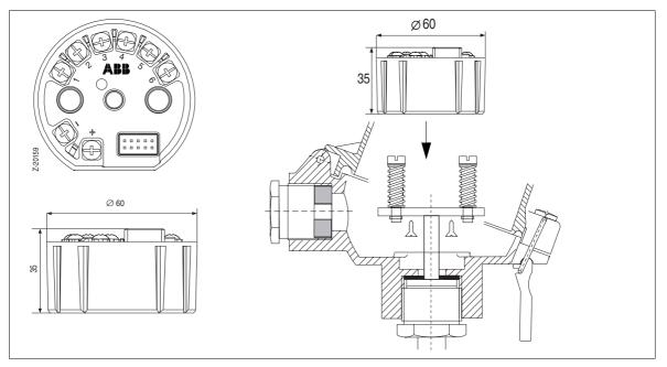
Fig. 3-1 Mounting the transmitter in the sensor head (all dimensions in mm) Mounting on a measuring inset with riveted bushes and springs (e.g. BUSH connection head) The measuring inset and transmitter are seen in the illustration rotated by 90°.
