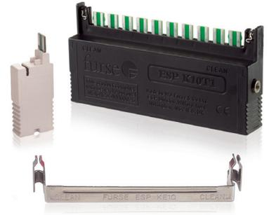
Combined Category D, C, B tested protector (to BS EN 61643) suitable for use on ten line LSA-PLUS disconnection modules to PBX telephone exchanges, ISDN and other telecoms equipment with LSA-PLUS disconnection modules. For use at boundaries up to LPZ 0 to protect against flashover (typically the service entrance location) through to LPZ 3 to protect sensitive electronic equipment.
