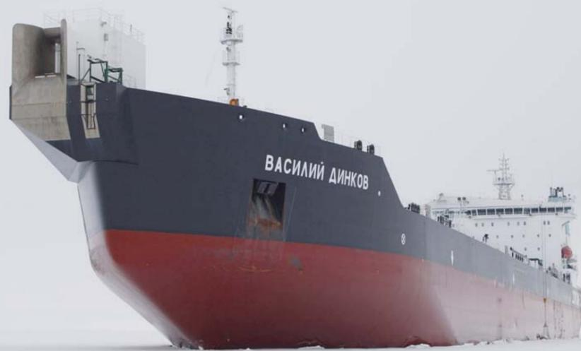
Sovcomflot's Arctic shuttle tanker *MT Vasily Dinkov* and her sister vessels are equipped with 2 x 10 MW Azipod VI propulsion systems.
