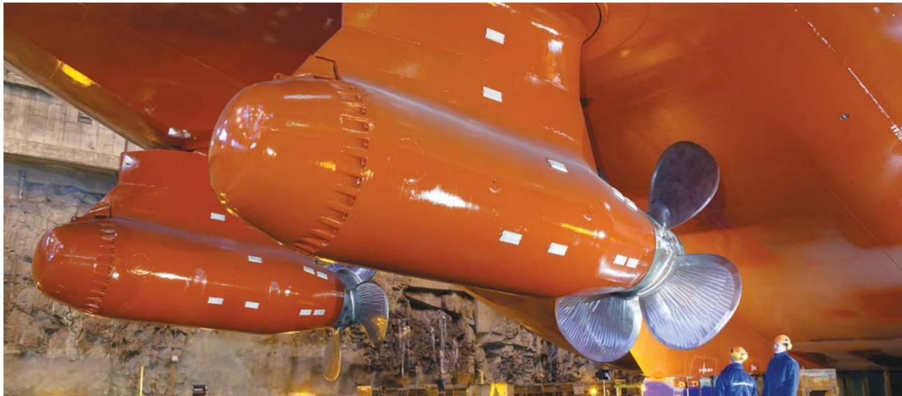
Azipod VI propulsion units are presently supplied for the power range from 1.5 to 17 MW.
