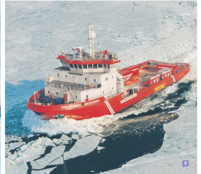
1. *Newbuilding* – icebreaking PSV. 2 x 6.5 MW Azipod propulsion. Owned by Sovcomflot, and built by Arctech Helsinki Shipyard.
