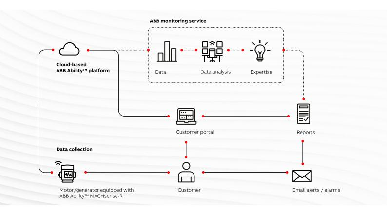
01 ABB's condition monitoring solution for HV motors and generators: ABB Ability™ MACHsense-R transmits data to a secure cloud. Algorithms analyze the data and convert it into meaningful information, which is sent to a dedicated web portal.
