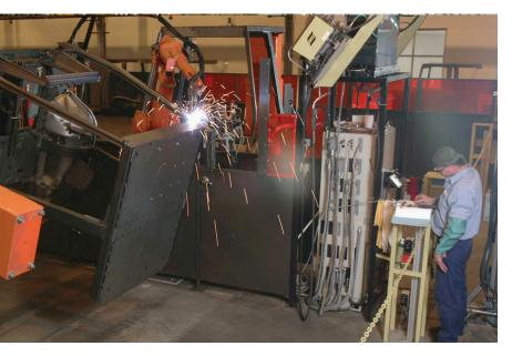
Based in Minnesota, Crenlo is an expanding specialist manufacturer producing rollover protection cabs for off-road construction equipment. Thanks to RobotStudio, ABB's offline rogramming software, the company was able to program its robots while its new plant in South Carolina was being equipped, thereby securing a prestigious order from Caterpillar.
