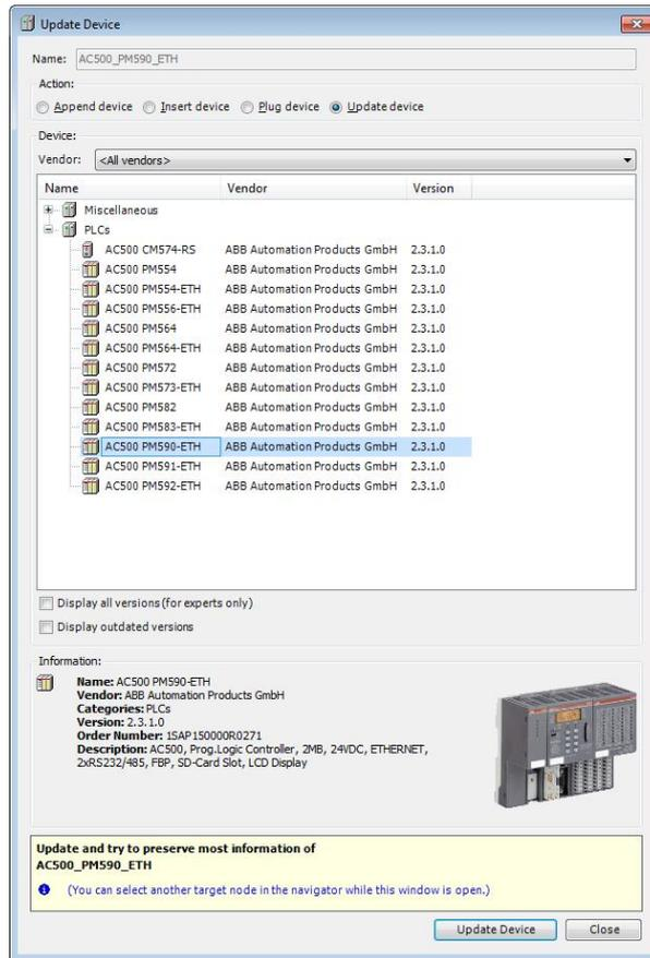
All sub nodes below the selected AC500 PM are automatically updated to the latest version 2.3.X in the device repository. The device update result is shown in the Message Window.
