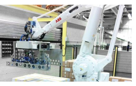
Barry Callebaut, the world's largest manufacturer of cocoa and chocolate products, recognised that a significant increase in operational efficiencies could be achieved through the installation of a robotic palletising system at its Banbury plant.
