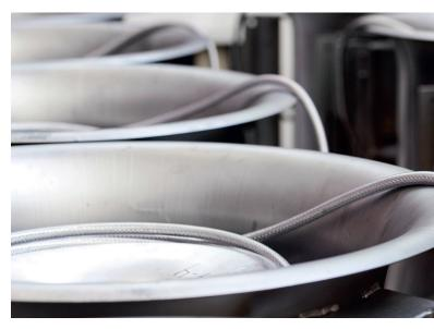
01 Paintfree solution eliminates the risk of paint chipping off and causing a food safety hazard.
