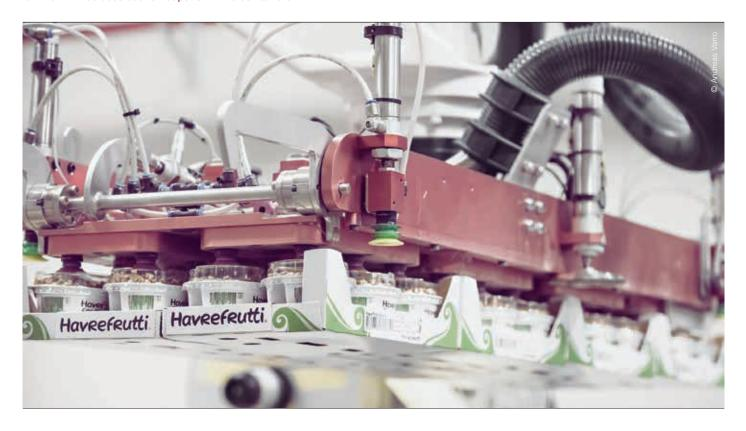
When a pallet is full, the robot changes function and uses the gripper to lift the new pallet into place. The robot can fill one pallet in 10 minutes, corresponding to a total of 8,500 products an hour.
