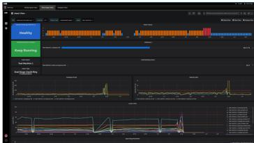
02 AssetInsight is a fully integrated condition monitoring system that gathers and integrates information from electrical, vibration and process equipment, devices and telecom and IT systems to enable a path
