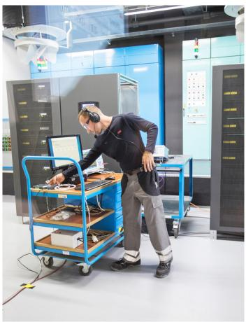
In addition to accommodating testing at 400 VAC, and standard voltages for Europe and other IEC markets, the facility can be adapted to perform tests at 208 VAC and 480 V, typical for the North America area and other UL markets.
