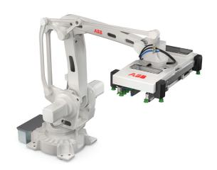
The FlexGripper - Vacuum is a simple plug-and-play extension to the ABB IRB 460 or IRB 660 palletizing robots. For maximum palletizing efficiency, the gripper can handle 40 kilograms and up to 10 products at the same time.
