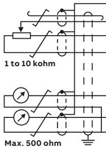
Default factory I/O connection diagram: Macro ABB standard
