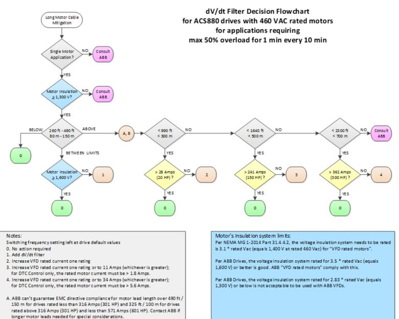
B. ABB considers motor leads over 490 ft or 150 m to be equivalent to a dV/dt filter
