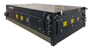
The BORDLINE® M80 DC static converter is a compact, rugged unit developed to feed auxiliary services of the metro.
