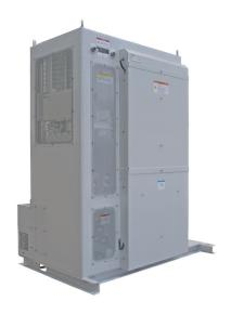
BORDLINE® M130 AC converts the power from the 25 kV / 50 Hz line into 415 V<sub>AC</sub>, three-phase auxiliary power for running auxiliaries of rolling stock applications.
