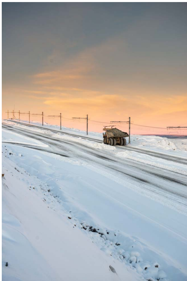
Figure 3. Boliden began trolley testing for ultra-class haul trucks at the Aitik opencast mine in Northern Sweden in late 2018. Photo courtesy of Boliden – photo by Mats Hillblom.
