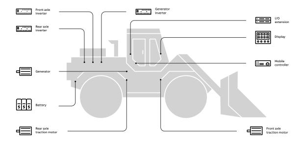
03 The ABB e-drivetrain, including e-mobility motors and HES880 drives, in use by Epiroc, for the global mining group's second-generation battery powered vehicles.
