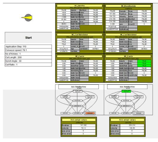
Initially ensure the master encoder is stationary (there is a small visualization to show the current position and speed of both the master and knife axes at the bottom of the screen). The axis should then enable and home automatically when the Start button is pressed (providing there are no errors). To reset an error condition deselect and reselect the Start button if required
