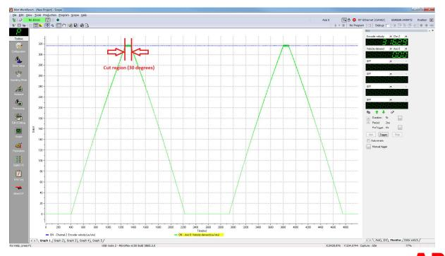
With the longer cut length the knife axis has to slow to a stop, dwell for a short time and then reaccelerate up to the synchronous material speed for the start of the cutting region.
