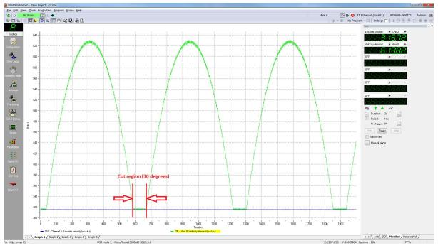
It can be seen that the knife velocity matches the master velocity for a period equal to the specified knife sync angle. With the default settings (i.e. a cut length of 200mm) the knife has to speed up in between cuts. The screenshot below now shows what happens if the cut length is increased to 800mm...
