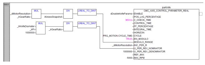
CYCLE is set to a constant with a value of 2ms to suit the EtherCAT cycle time set in our Automation Builder device configuration. EN\_MODULO is set to true because the axis continually runs in one direction and wraps every rev of the knife.
