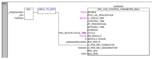
CYCLE is set to a constant with a value of 2ms to suit the EtherCAT cycle time set in our Automation Builder device configuration. EN\_MODULO is set to false because although the axis continually runs in one direction the application code always shifts the axis position backwards after every cut so it never effectively gets any larger than the maximum cut length.
