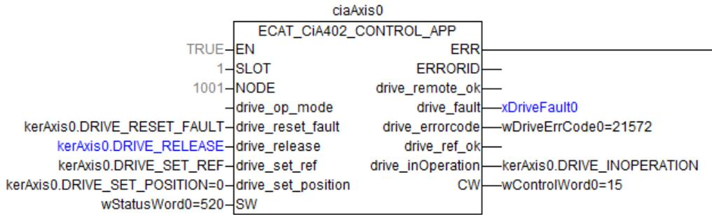
The drive\_fault output will become TRUE in the event of a drive error occurring. At the same time drive\_errorcode will report the appropriate DS402 error code. The table below (extracted from the Mint Help file) shows the list of possible errors and their associated DS402 and Mint error codes...
