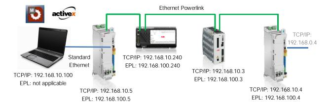
In our example network we have a NextMove e100 with 3 drives, a MicroFlex e100 and 2 x MotiFlex e180 (one operating as an EPL router) on an EPL network (one or both of these could equally have been MicroFlex e190 drives, but for this application note we will assume MotiFlex e180 drives have been used throughout). The TCP/IP addresses listed under the devices are the addresses as seen via the EPL router (entered in the NAT table).
