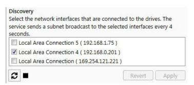
Once uploaded select 'Network' from the list of available options. The screenshot below shows the section from the 'Network' screen responsible for setting the drive's generic Ethernet address and subnet mask (the screenshot it taken from a MicroFlex e190 connection, this is identical for a MotiFlex e180).
