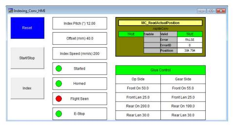
Once enabled the visualisation included with the PLC project provides the ability to "start/stop" the system. If the system is not started, indicated by a red 'led' mimic, it is not possible to index the axis. Once started operating the index button will either...
