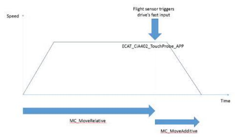
Motion is initially started using MC\_MoveRelative. The program loads the programmed pitch as the move distance for this block. If the flight sensor triggers the drive's fast digital input (input 1 in this case) during this movement then MC\_MoveAdditive is executed with the 'Distance' input parameter for this function block calculated to ensure the axis stops the programmed 'Offset' distance past the axis position when the fast input occurred....
