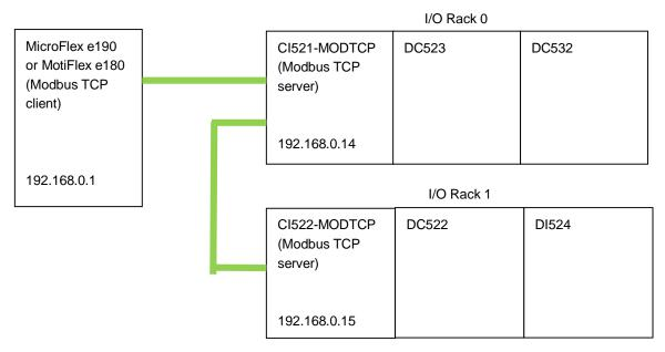
We will daisy chain the Ethernet cables between the drive and the I/O modules making use of the built in switch on the CI521 module, but it would be equally valid to create a star type Ethernet network using an additional switch between the drive and the I/O racks.
