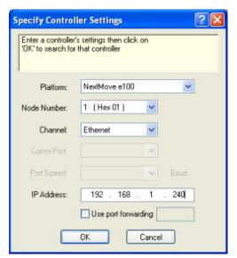
Enter the required information for the e100 device you are connecting to. The options for our NextMove e100 are shown on the left. Note: The node number drop down box has no affect when connecting to an Ethernet device. click ok.
