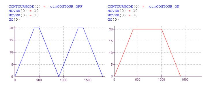
When a move is loaded into the buffer, the contour mode is stored as well, allowing some moves to be loaded with contouring turned on and others with it turned off. For example:
