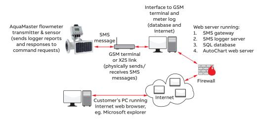
ABB's AquaMaster 3 electromagnetic flowmeters include GSM-SMS radio technology, enabling up-to-date information to be remotely collected from anywhere around the world.
