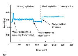
In the presence of dense foam, the LLT100 will return the level of the top of the foam. However, the LLT100 is not confused by foam and the measurement is not lost or erratic.
