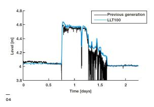
Furthermore, the LLT100 was also installed next to a competitor's ultrasonic sensor for reference. The results also show the stability of the LLT100 output, unaffected by the daily temperature changes: the LLT100 line is straight when no filling occurs, while the competitor's product line shows a daily oscillation.
