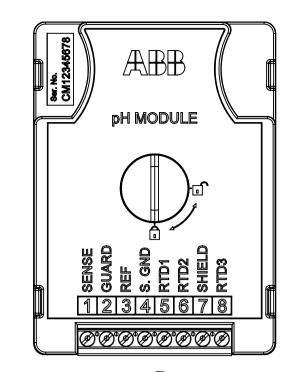
OUTPUT PARAMETERS - pH Voc(Uo) = 11.8Vlsc(lo) = 11.8mAPo`= 36mW Ca(Co) = 1.5uFLa = 1H
