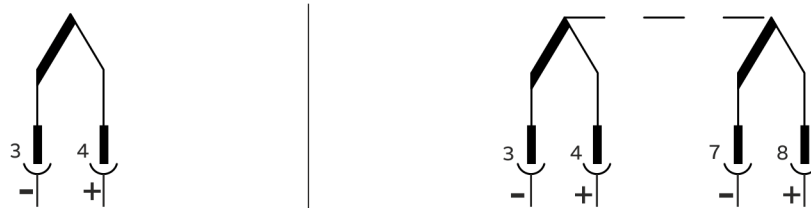
Figure 32: Thermocouple as single sensor or double sensor
