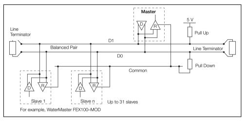
Fig. 2.1 Typical MODBUS RS485 2-Wire Network Installation
