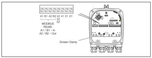
Fig. 3.1 WaterMaster FEX100-MB RS485 Backplane Wiring Terminal Connections to MODBUS Network
