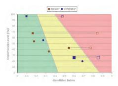
The categorization of plant substations chart, in the Importance/ Condition matrix, gives an overview of the current condition of each substation on the plant, linked to its importance.
