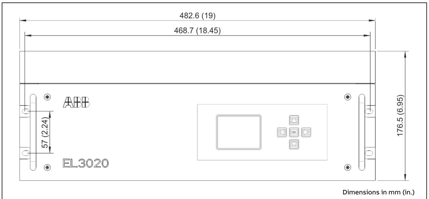
Note: Only the front view of the housing (with its height differing from the standard dimension) is depicted in this dimensional drawing. Refer to the dimensional drawing on page 42 for other views and dimensions of the 19-inch housing.
