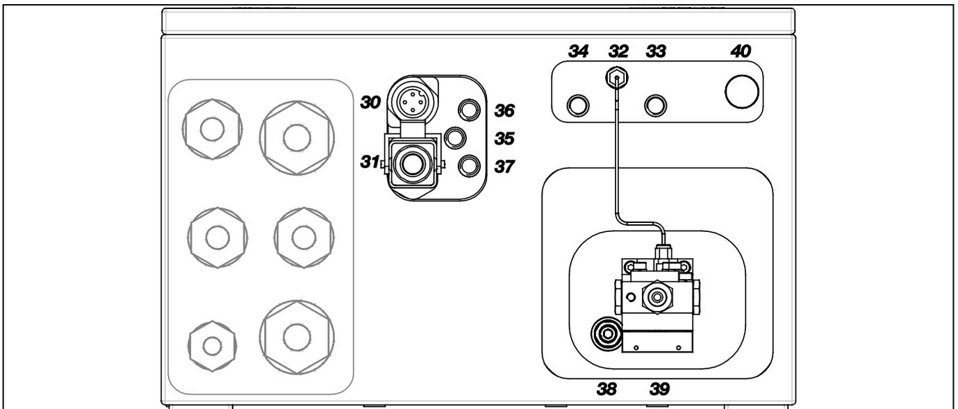
**30** Power supply AC 115 V or 230 V for heating of detector and sample gas inlet (4-pin male plug, connection cable included in scope of supply)
