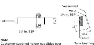
Customer-supplied holder nut slides over sensor and threads onto tank bushing
