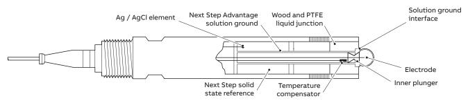
ABB TB(X)5 series sensor construction
