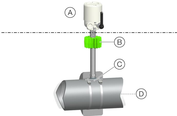
Figure 13: Temperature sensor fastening 90° to the piping with Energy Harvester
