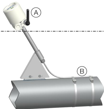
Figure 12: Temperature sensor fastening alongside the piping
