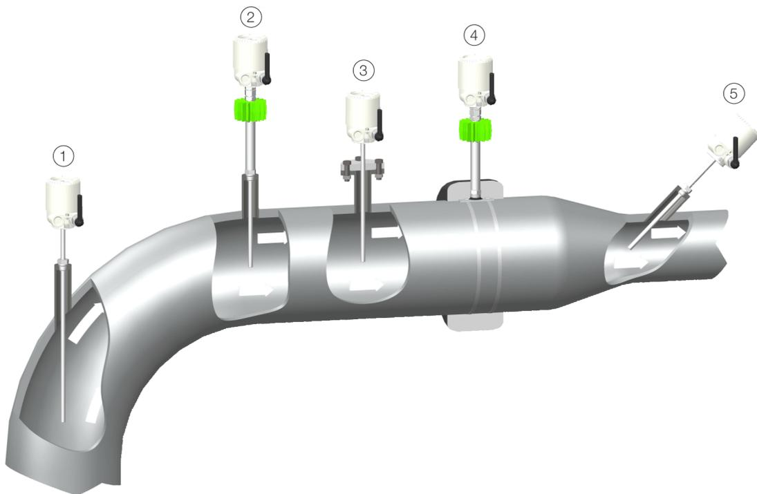
Figure 5: Installation positions
