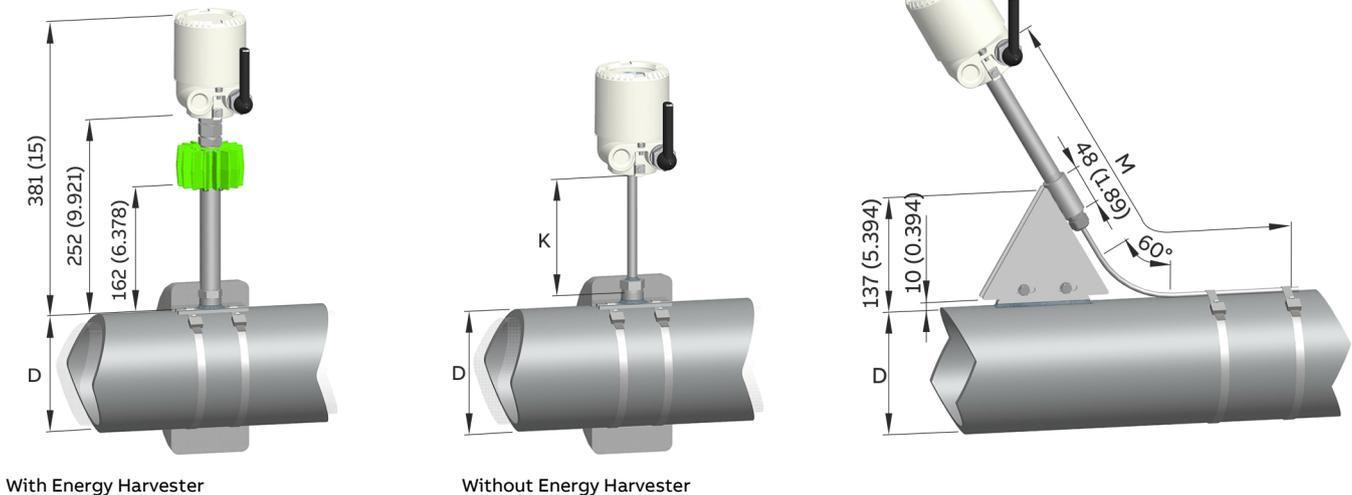
Figure 8: Sensor fastening 90° to piping / alongside piping
